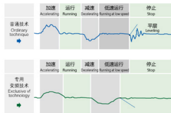
加减速曲线对比 A comparison of accelerating and decelerating curves
